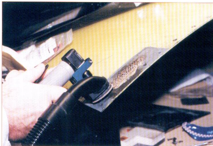
A small burn-through area on a carbon fibre/epoxy door requires sanding to complete repair on the US Space Shuttle. (Source: FlightSafety.)
